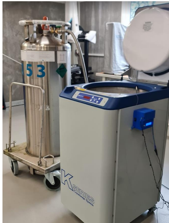
Figure 11 – Cryogenic freezer 10K-M505K and Liquid Nitrogen vessel.
