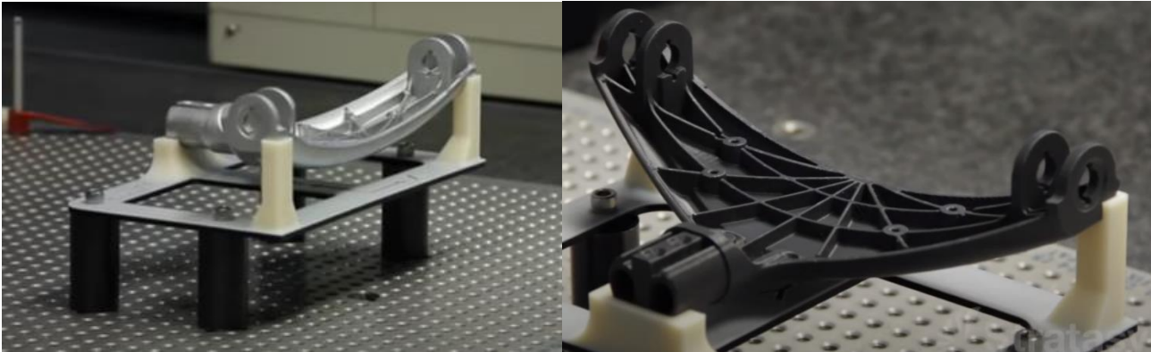
Figure 8.2-2 Stratasys AM fixtures [17]
