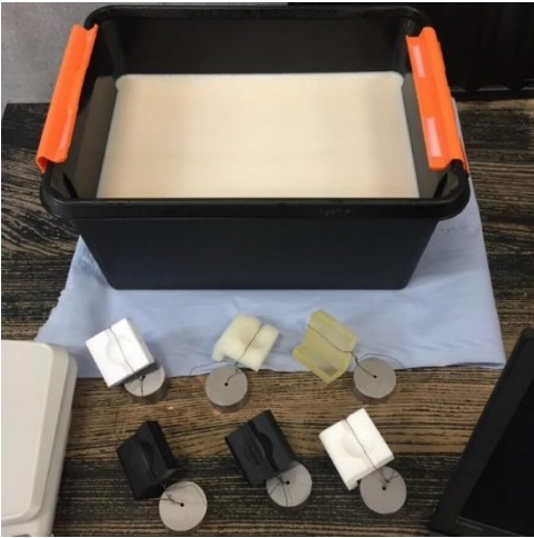
Figure 8.1-1 UPUV - 3D print fixtures and tools (P654) absorption test setup
