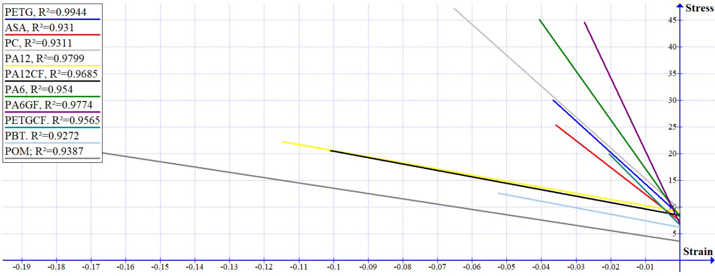
Figure 10.2-4 Compressive modulus regression
