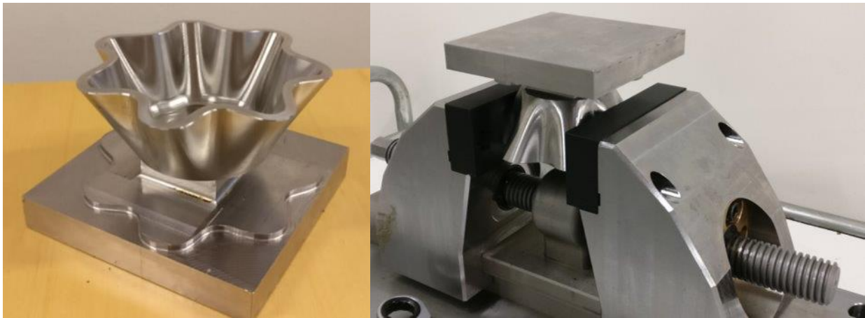
Figure 8.2-3 “Demo 7 lobe bowl” Complex jaw fixture UPUV - 3D print fixtures and tools (P654)
