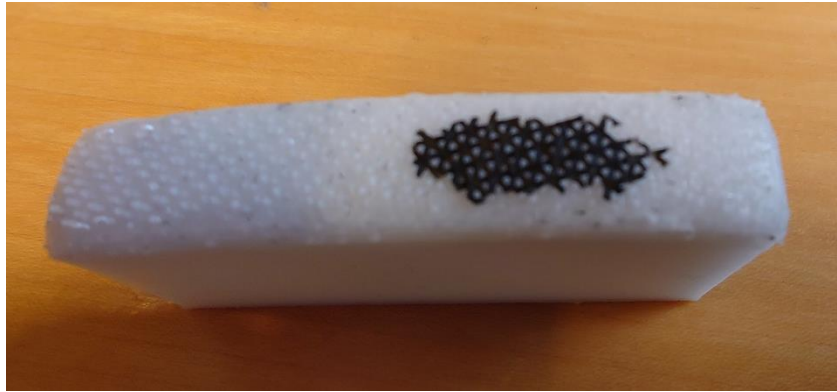
Figure 10.6-2 3D printed POM using PETG and PA6 raft
