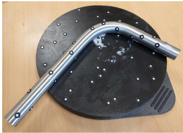
Figure 10.7-7 VOLA 3D scan using spray and markers
