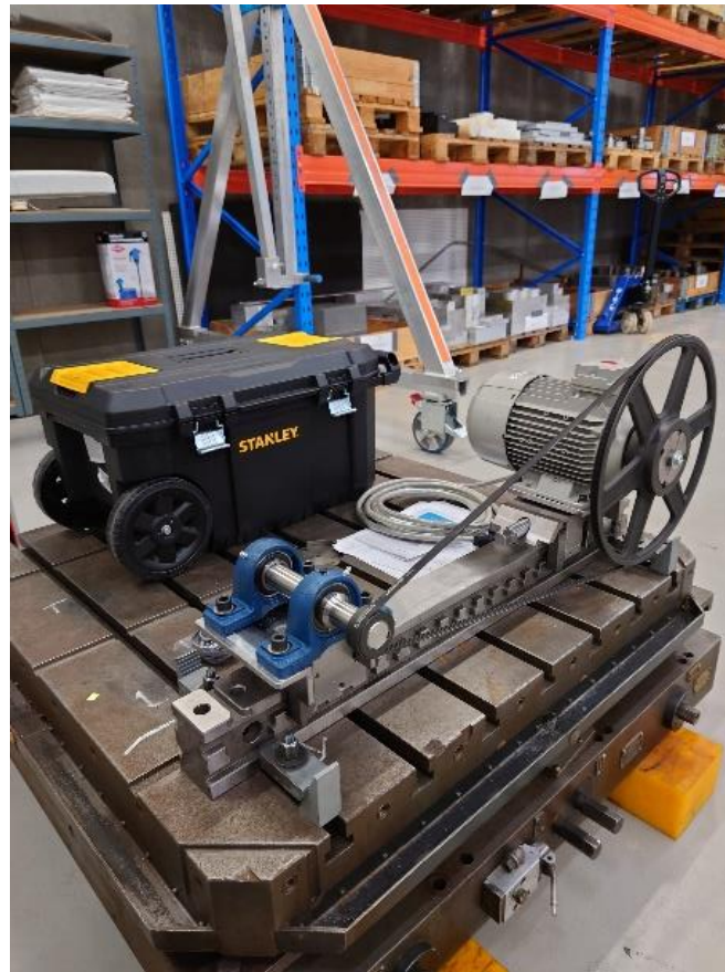
Figure 24: The test rig used at DAMRC to verify the implemented envelope analysis
