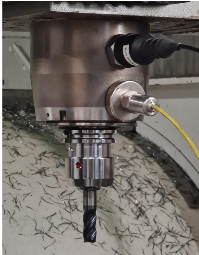
Figure 37: Accelerometer placement on the DMU.
