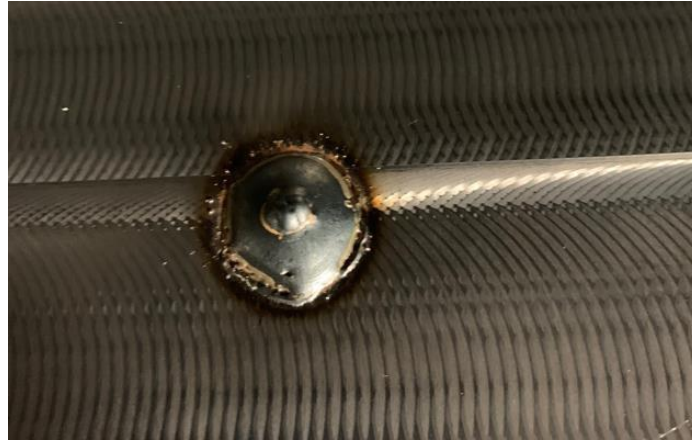
Figure 7. First welding attempt in CNC-center
