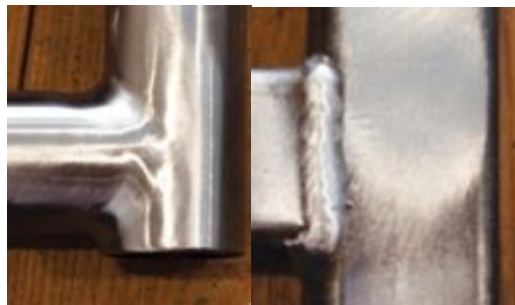
Figure 6. An example of a good weld where the joints do not show any sign of welding (left). An example of a bad weld where it has been partially dressed and the spatter removed (right).
