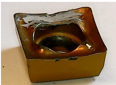
Figure 110: Super Duplex – Tools – LN2 – Drilling.
