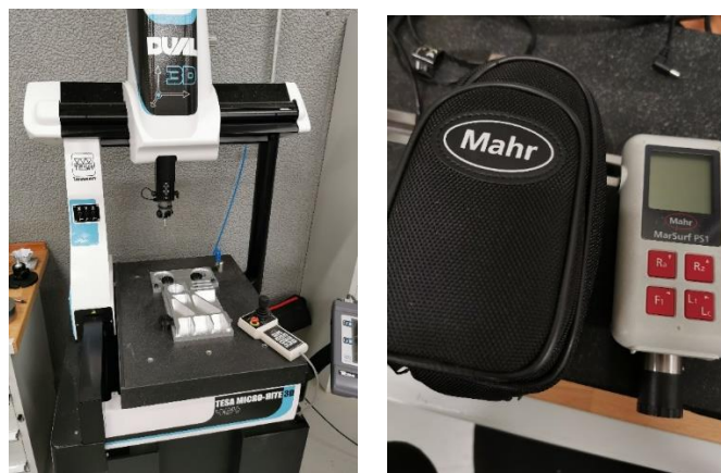
Figure 38: Left, TESA CMM surveyor. Right, Mahr roughness meter
