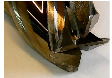
Figure 59: Aluminium – Tools – LN2 – Scrub.
