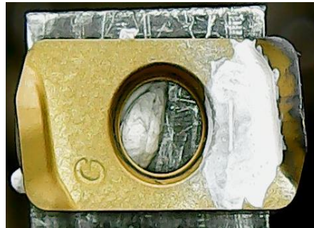
Figure 117: Super Duplex – Tools – LN2 – Scrub.
