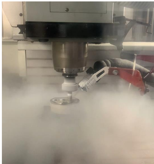
Figure 101: Super Duplex – LN2 – Process.
