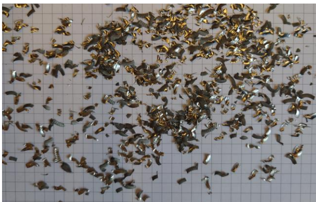
Figure 88: Super Duplex – Chips – O/W - Scrub Macro View.
