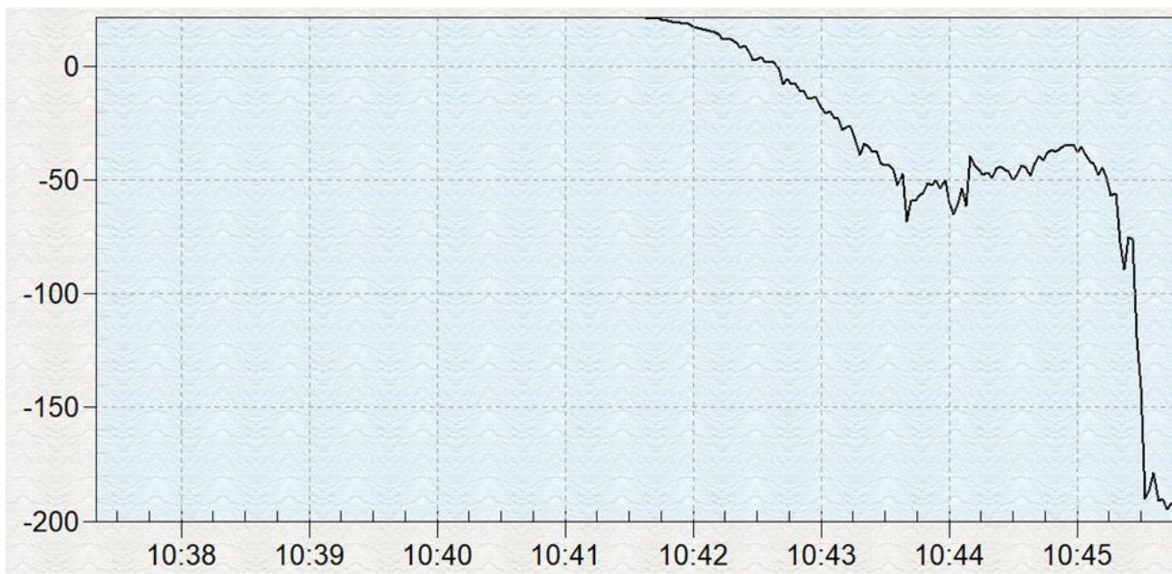
Figure 141 – Temperature chart resulting of test with R390-016A16-11L 800 RPM– 5 Bars of LN2.
