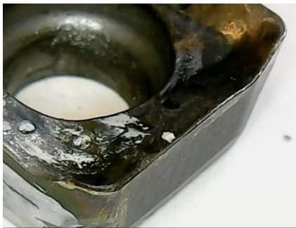
Figure 113: Super Duplex – Tools – LN2 – Drilling.
