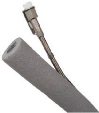
Figure 2 - First iteration LN2 supply system for LN2 turning project.
