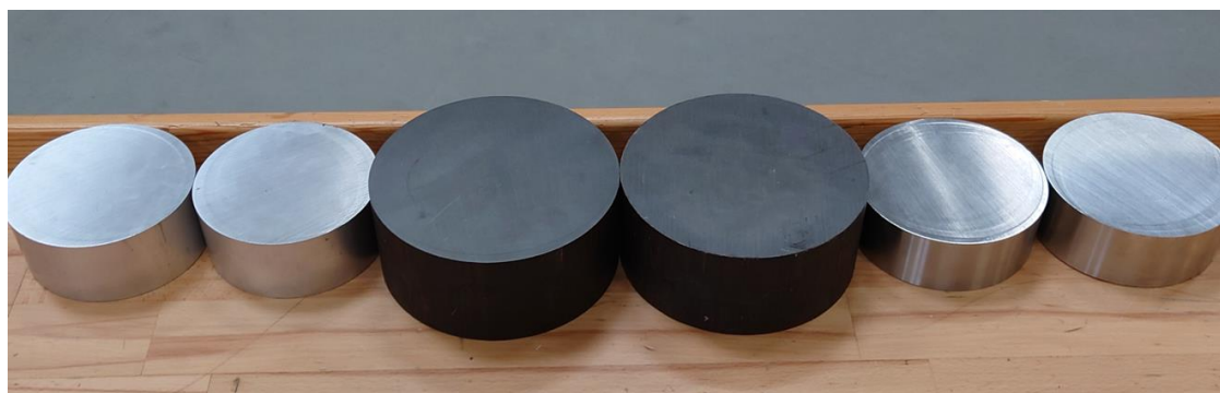
Figure 16 - Test samples materials - AW6026 in the left, EN-EJS-500-7C in the middle, SAF 2507 in the right.
