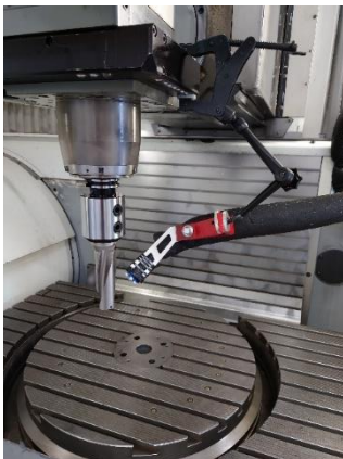
Figure 35 - Liquid Nitrogen delivery system.
