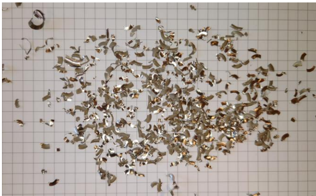
Figure 106: Super Duplex – Chips – LN2- Scrub Macro View.
