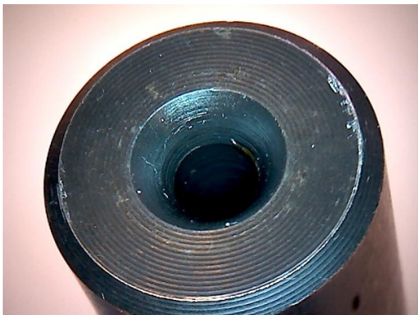
Figure 136 – Coolant inlet hole R390-016A16-11L.
